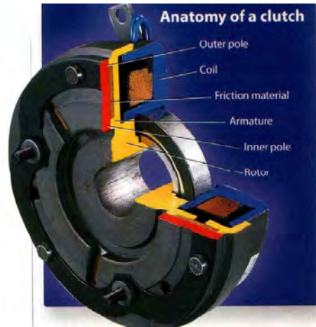
Figure 14: Schematic of an electromagnetic clutch [61]
